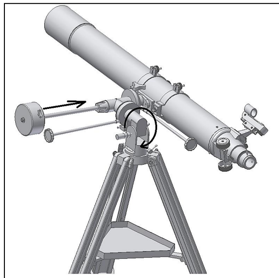
Figure 10. Balance the telescope tube R.A. axis.
